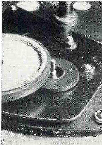
Fig. 1. Enlarged view of the motor shaft and idler wheel of a typical 33 1/3 rpm record-player motor. See text for details on how author converted unit for 45 rpm.
