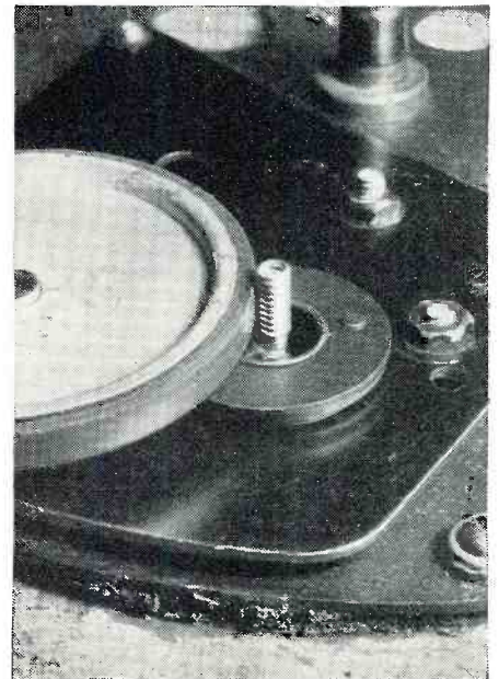
Fig. 2. Same motor as Fig. 1 with a copper wire coil spring slipped onto shaft to raise turntable speed to 45 rpm. Thickness of spring wall prevents turntable "wow".
